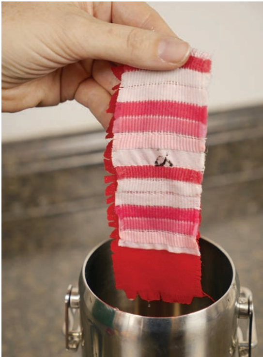
Stained Multifiber from Rotawash Container
